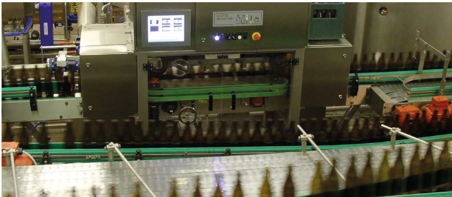
Bottling line equipped with a bottle inspection system
