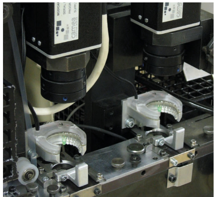
System illumination units
